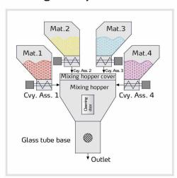
Motor starts after receiving the signal from the control box. And materials in hopper will drop into the screw through screw rotating driven by the shaft coupler, which will be conveyed to the base by screw after it receiving the squeeze from the screw as to achieve accurate metering and material conveying purpose.
